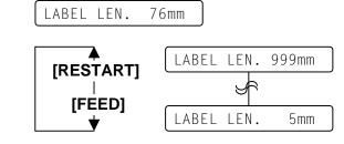
**[FEED]** key: Pressing the **[FEED]** key one time causes a -1 mm change, up to 5 mm.
